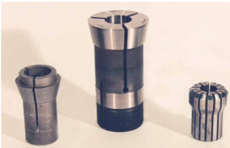
The three basic styles of collets (left to right): push, draw and compression.
