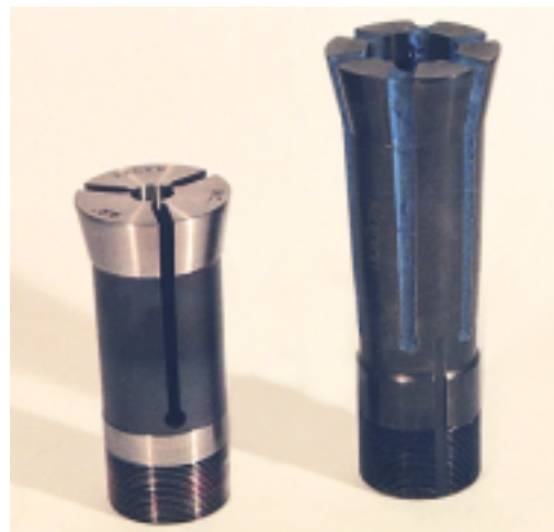
The most common draw collet is the C-type, such as the standard 5C (left) and the special 5C with caulked slots.
