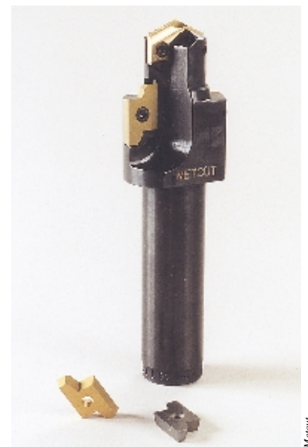
A double-effective port tool accepts one spade-blade insert for drilling the hole and two form inserts for creating the port's form and face.
