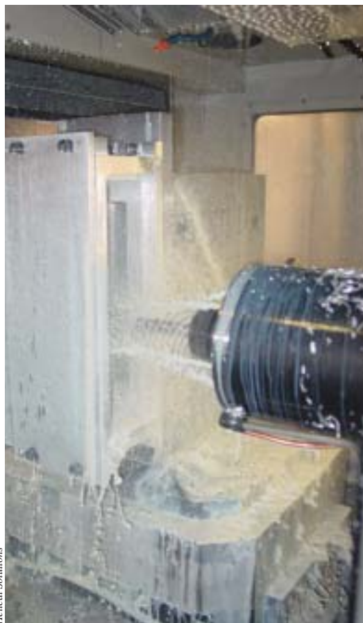
P/M endmills are effective for roughing all ferrous and nonferrous materials.
