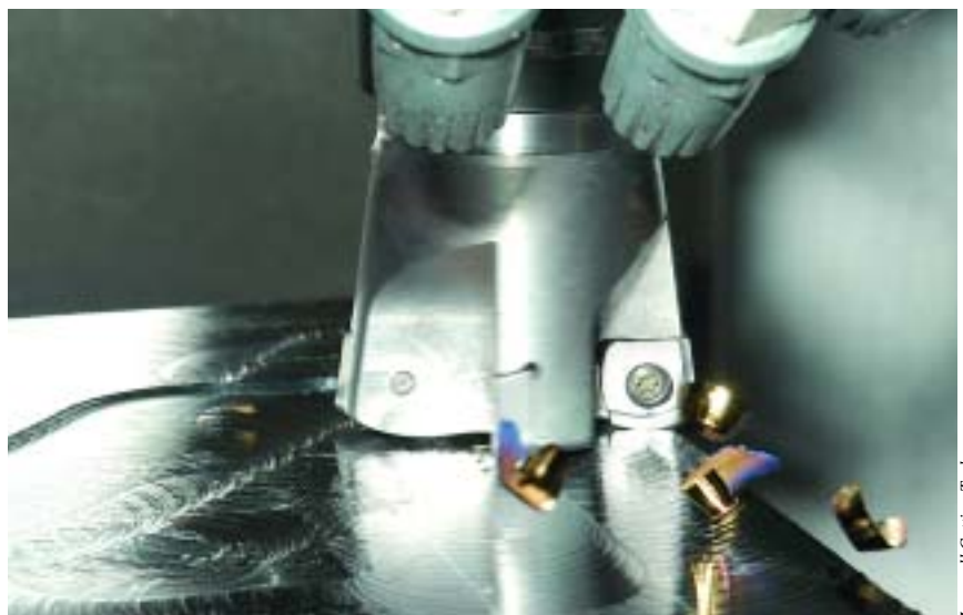
With a large edge radius and drafted periphery edge, Form-MasterSpeed high-feed inserts applied at a shallow DOC when milling can help control chatter by redirecting forces into the machine spindle.
