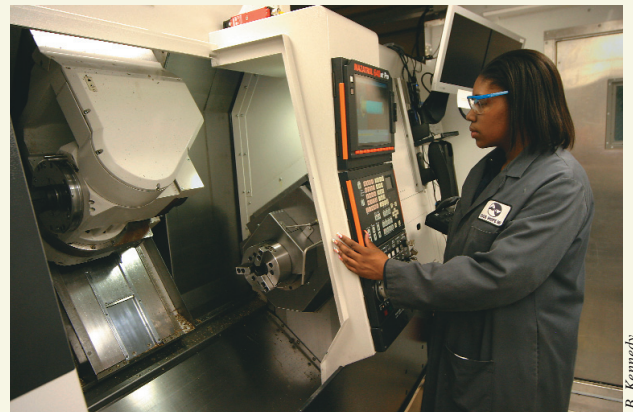
In a RMS currently being used for training at Focus: HOPE's Center for Advanced Technologies in Detroit, engineering candidate Shakemma Taylor works with the CNC of a Mazak multitasking lathe.
