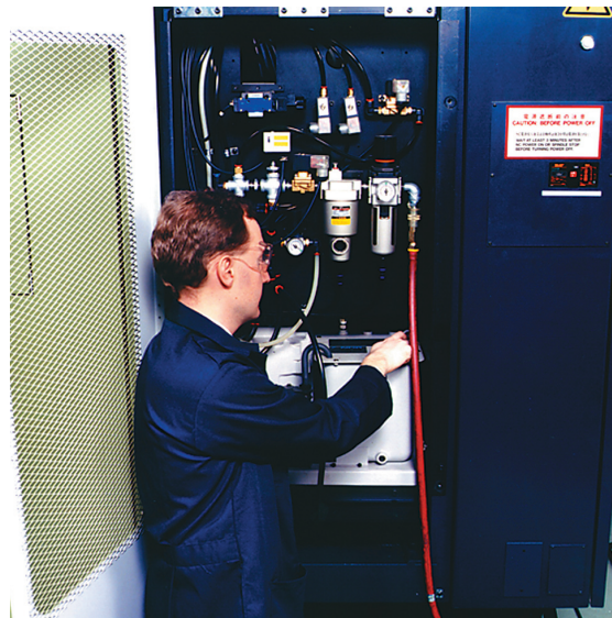
Makino's V55 vertical machining center is designed for easy access during routine maintenance.
