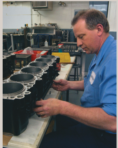
Technician Karl Bausman works with the water-jacket plumbing on part of a V-12 Merlin engine.
