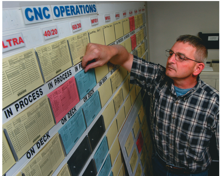
Job coordinator Bob Gadigian at Roush Machining Services' whiteboard, which employs color-coded cards to indicate the urgency and status of each job in the production schedule.
