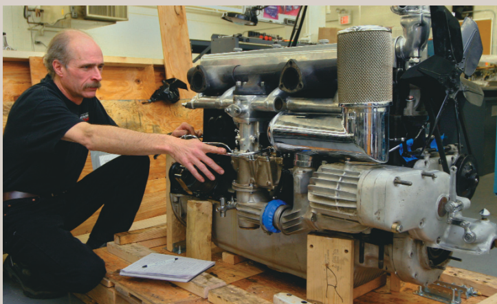
Vintage engine builder Fred Burkhart displays a straight-eight engine from a 1937 Mercedes 540K.
