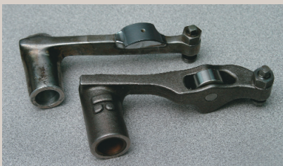
New rocker arms with roller ends (foreground) designed to replace arms with sliders for the V-12 Merlin engine.
