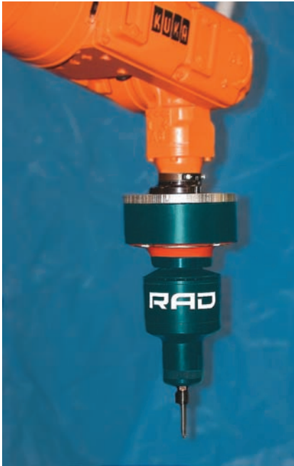
The Ultiburr deburring tool is compliant in the X, Y and Z axes.
