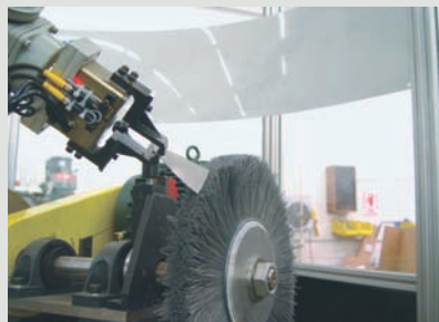
A robot carries a turbine blade to be deburred by a nylon abrasive filament brush from Weiler.
