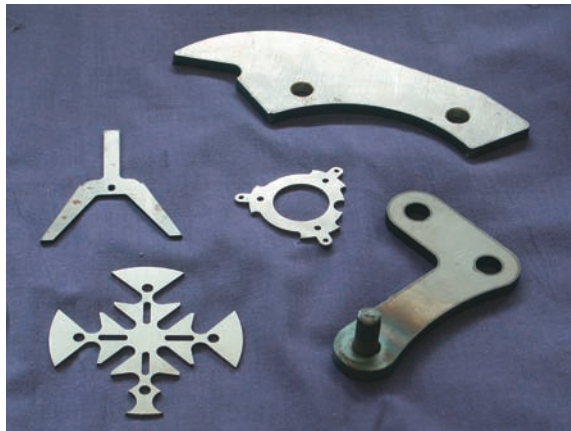
Various 2-D sheet metal parts cut at Tesko with its laser cutting machine.
