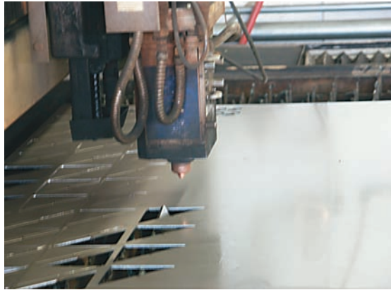
Tesko's 2-D laser cutting machine cuts 2-D sheet metal parts.
