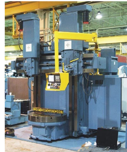
Daniluk took a mechanically worn out 1954 Giddings & Lewis vertical boring mill (top) and transformed it into a 2005 machine.
