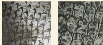
A Bridgeport mill being rebuilt at S.T.K. (top left) and a completed version. Bottom: When rebuilding a Bridgeport, S.T.K. scrapes and flakes worn way surfaces (left) to achieve a like-new condition.
