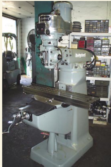
A Bridgeport mill being rebuilt at S.T.K. (top left) and a completed version. Bottom: When rebuilding a Bridgeport, S.T.K. scrapes and flakes worn way surfaces (left) to achieve a like-new condition.
