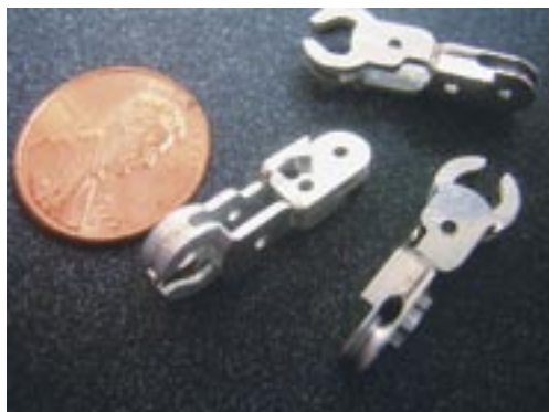
This gripper part demonstrated how EIGERlab’s tabletop microfactory is capable of machining, inspecting, assembling and welding.
