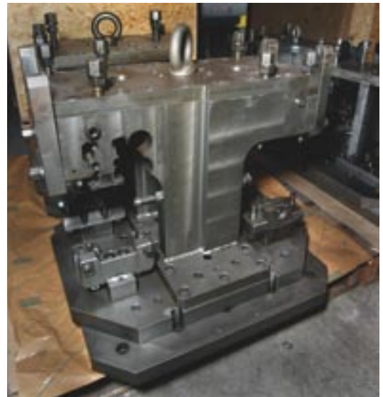
By changing the tombstone fixture and subplate as a unit when tooling up for new parts, AUMA significantly reduced setup times.
