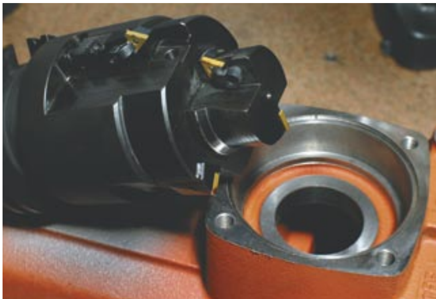
Multifunction cutter and the cast iron housing it was designed to produce.
