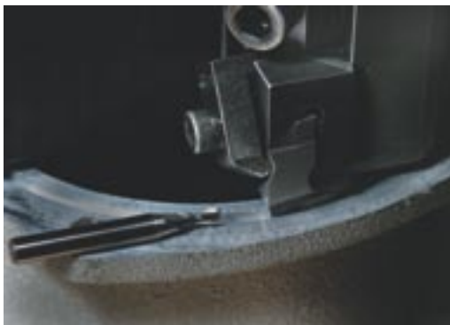
A grooving insert fitted in a multifunction cutter replaced a 2.5mm-dia. endmill that required two passes to interpolate a
