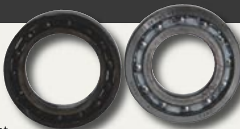
All bearings must be kept in the best condition possible to achieve the desired results. The bearings on the left are no longer usable; those on the right are new.
