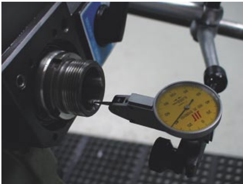
Note the location of the indicator and base. Mounting the base directly to the holder helps avoid an inaccurate reading.
