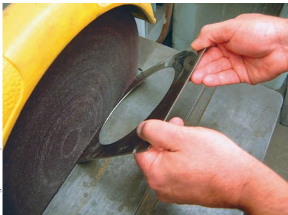
Deburring the edges of thin plates can be dangerous if the support table of a disc sander is used, because the plate can get sucked into the small opening between the table and the disc. This pulls the plate and the machinist's thumbs into the rotating disc.
