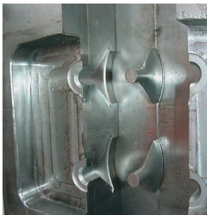
This mold's core is an example of a lofted surface.
