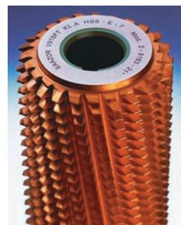
A gear hob's Nd:YAG laser-marked end.
