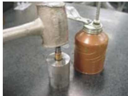
Using hydraulics to remove a bushing from a blind-hole.
