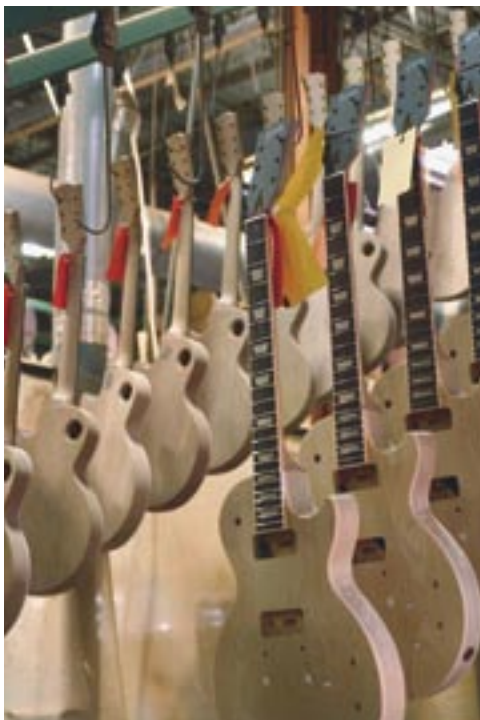
Guitars hang for 4 to 5 days to allow the lacquer to fully dry.
