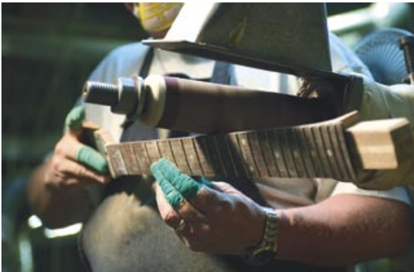
A veteran Gibson craftsman hand-works the neck on a Les Paul, a process called "neck rolling."
