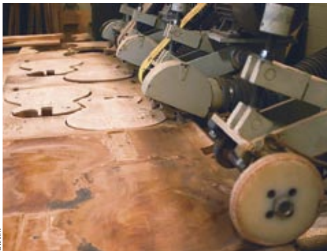
The tracing mill, or “guitar copier,” rough-planes bodies of the Les Paul.
