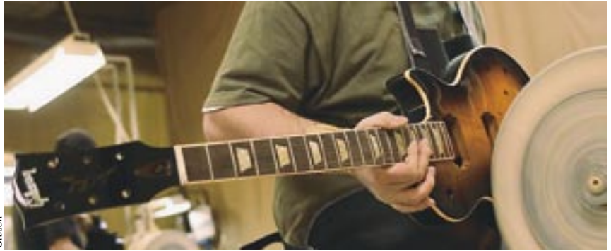
Les Pauls are renowned for their lustrous finish, a result of six coats of lacquer and a buffing process.
