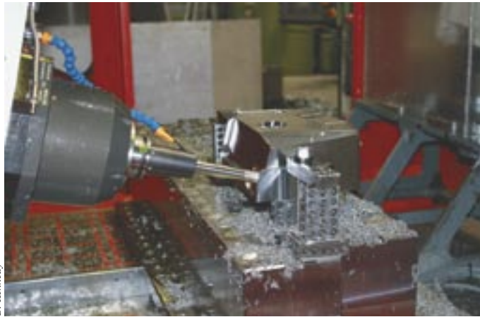
Five-axis machining permits manufacturing of some molds in one setup, streamlining the entire manufacturing process.
