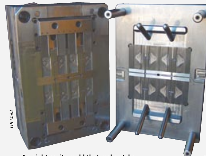
An eight-cavity mold that makes tabs used to attach a metal D ring to the knee brace.
