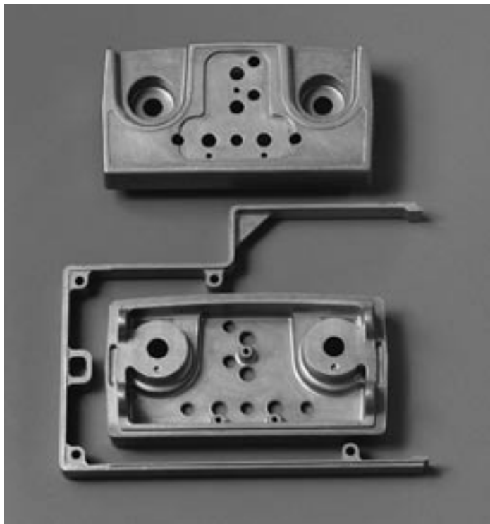
To fill a special customer request, CNC Technologies machined a delicate spacer and two-outlet end cap out of magnesium for a wireless-communication case.
