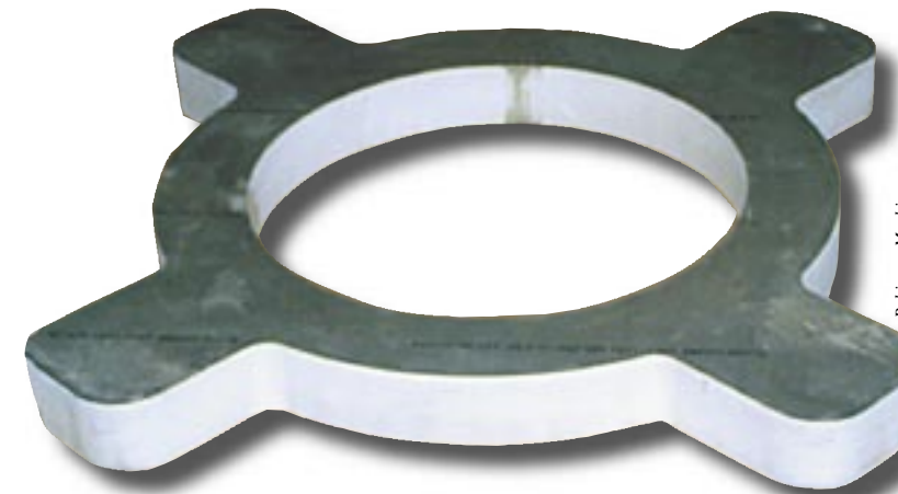
A 2 1/4"-thick aluminum part cut on an AWJ table.
