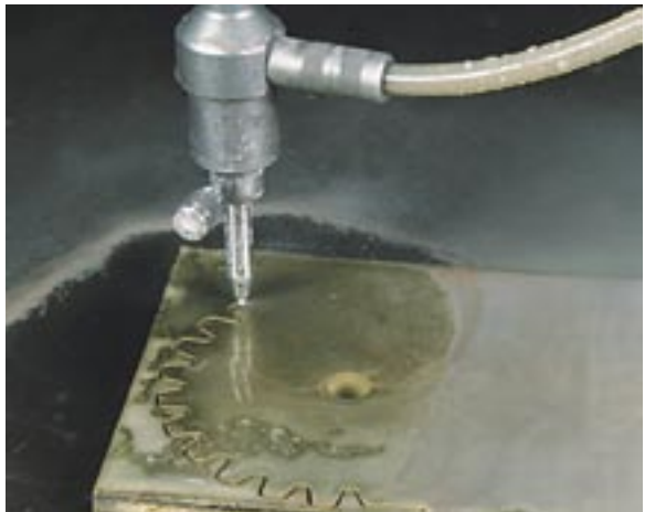
A gear being AWJ-cut from a brass workpiece.
