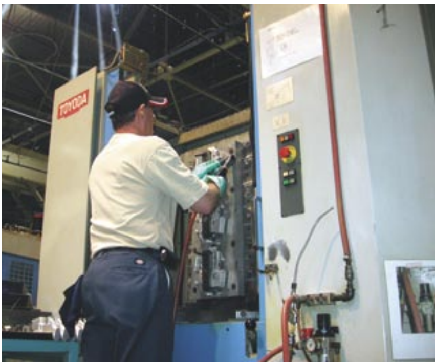
A Colt machinist loads a tombstone with M4 lower receivers.
