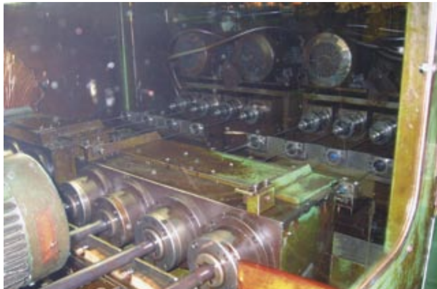
Each step in the gundrilling process begins with multiple 4,000-rpm drills cutting into raw gun-barrel stock rotating at a predetermined rate in the opposite direction. The operation is accurate to 0.0007".
