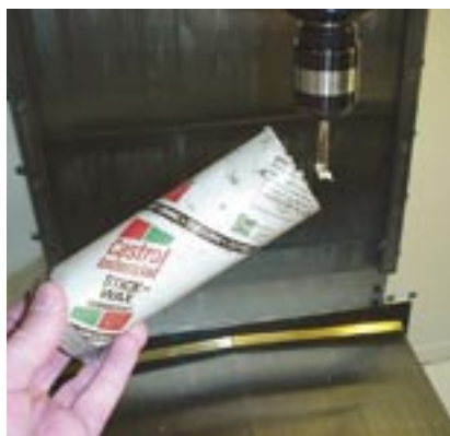
Stick wax lubricant adheres to a tap even under a coolant stream.
