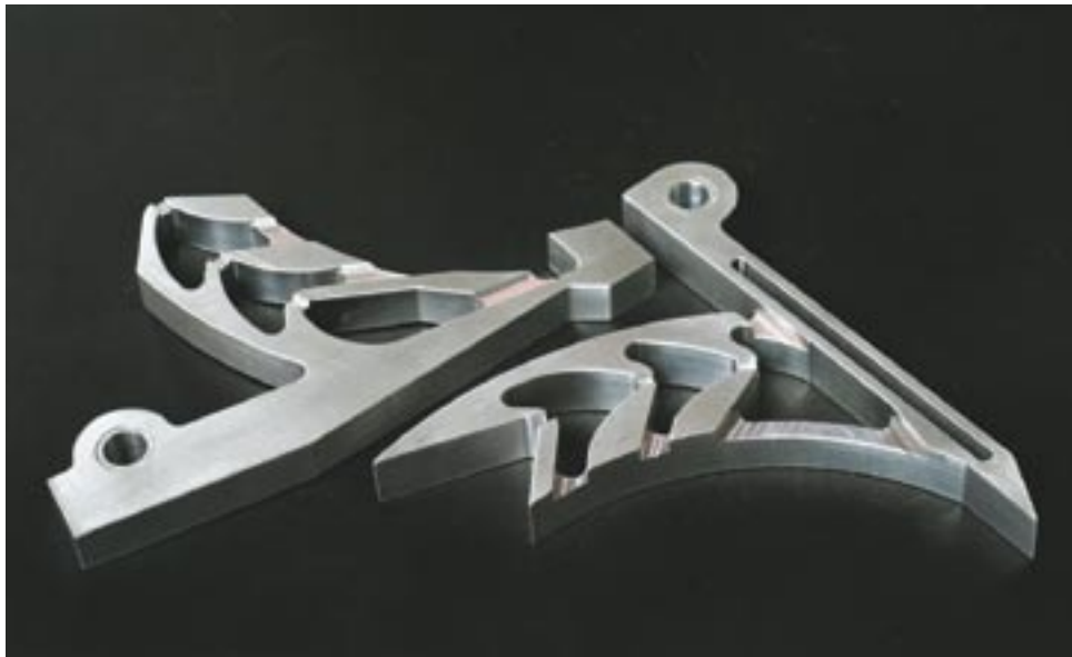
Falcone Precision Machine made aluminum test parts as a trial for a short run of brass components used in a P/M processing machine.
