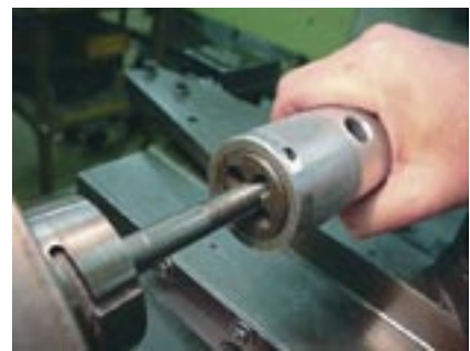
A die button mounted in a guiding jig is used to finish an external thread.
