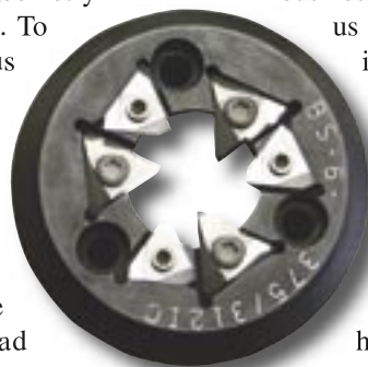
An F&F-designed thread whirling body tooled with three roughing and three finishing inserts.
