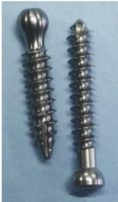
Examples of bone screws with whirled threads.
