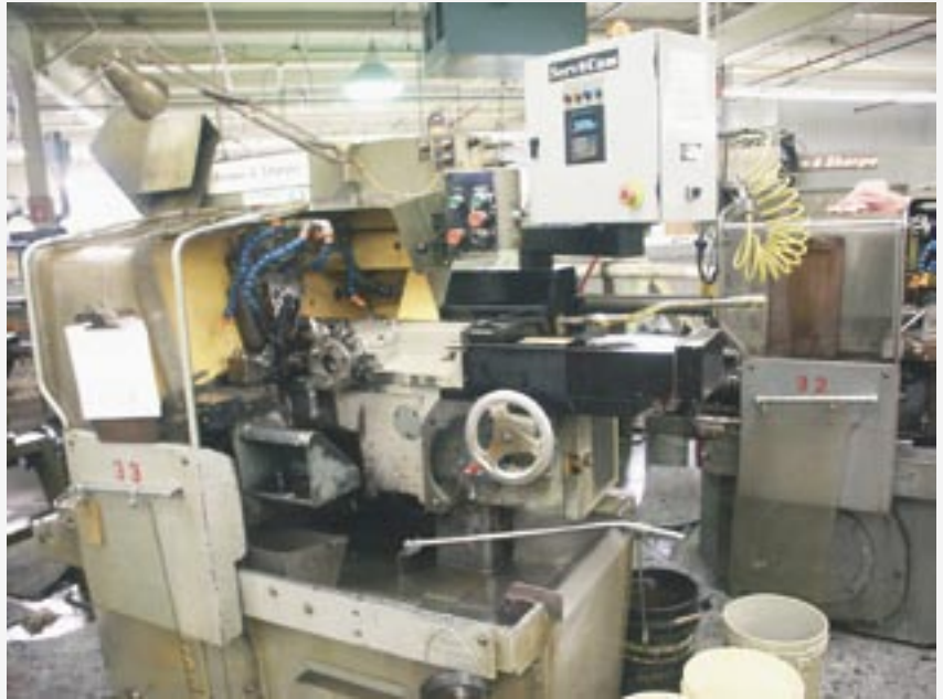
A Brown & Sharpe single-spindle screw machine retrofitted with ServoCam technology, which turns the critical turret-slide axis into a CNC ballscrew drive.
