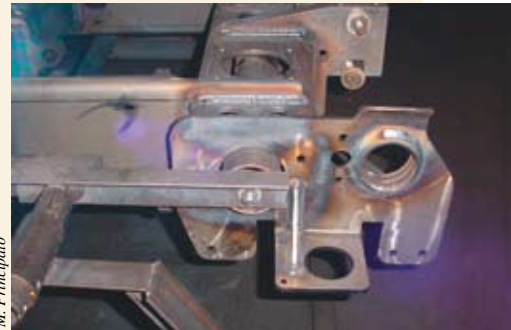
Weldment mounted to coaster train chassis.
