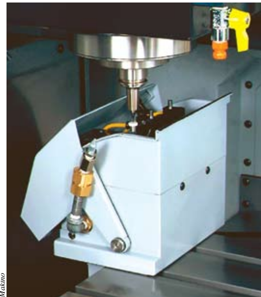
To accurately determine the position of the tiny tools applied in micromachining, Makino developed a hybrid automatic tool-length-measuring system that combines static low-pressure contact sensing with noncontact sensing performed while the tool is at operating speed, permitting submicron tool positioning accuracy during machining operations.
