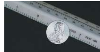
Produced as a test for a maker of coining dies for currency and tokens, this coin was machined on a Benchman MX VMC with a 0.001"-dia. endmill in a cycle time of 8 minutes.
