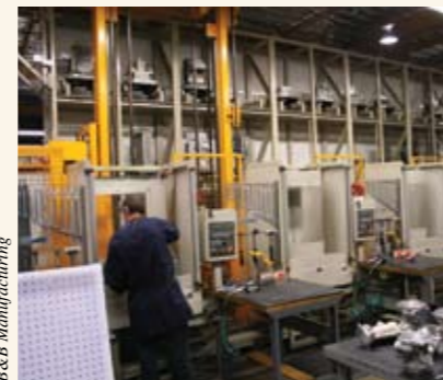
FMSes are best suited for small-lot repeat jobs. Preparing the jobs means creating part queues for the FMS. The queues are created at load/unload stations, placed in pallet storage racks—sometimes multiple-level racks—and moved to machining centers by a transport system, like the orange rail-guided vehicle pictured.
