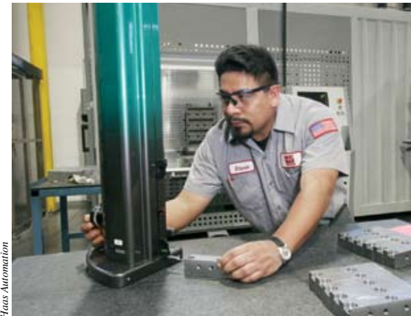
An FMS can make first-article inspection a task for a recurring job's first run only. With the setup remaining intact between runs, later runs could require only in-process inspection. Here, an FMS operator performs a routine, in-process inspection on parts machined in an FMS.
