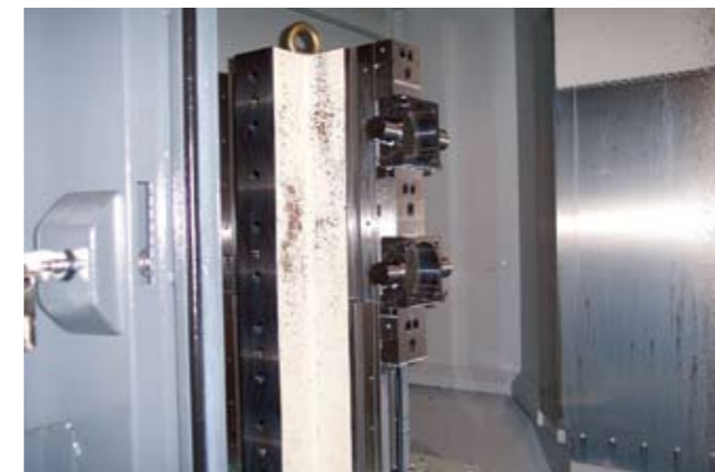
Tombstones are a common part of many FMSes and allow for machining many of the same part or machining of multiple part numbers within one machine tool.
