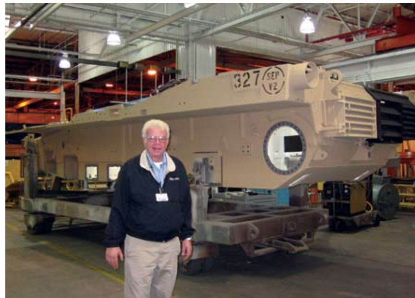
General Dynamics' Dick Sutliff with a freshly primed Abrams hull ready to join the assembly line.
