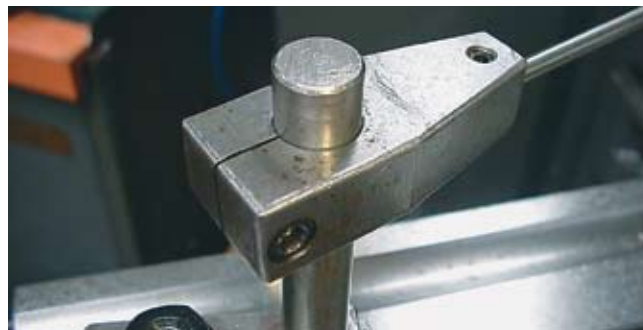
Flex-type bar clamps work well when there's enough weakness in the flexing area.
