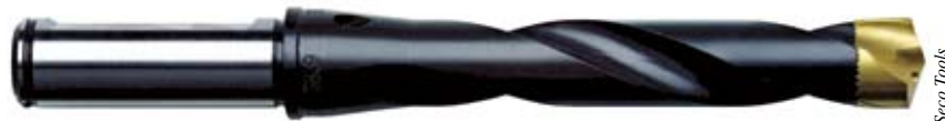
Seco Tools’ CrownLoc replaceable-crown drill employs a pull rod through the body that screws into the bottom of the crown, then pulls the crown securely into the body.
