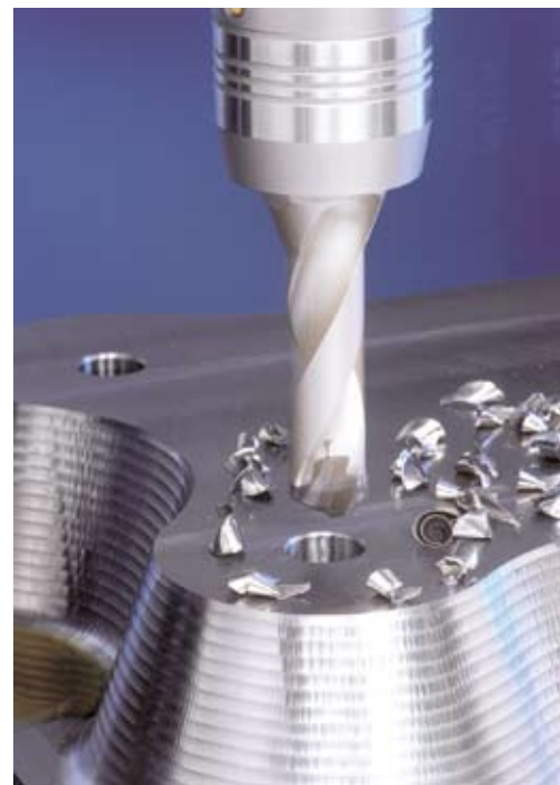
Iscar Metal’s replaceable-crown drill uses a key that grips and then twist-locks the crown onto the body.
