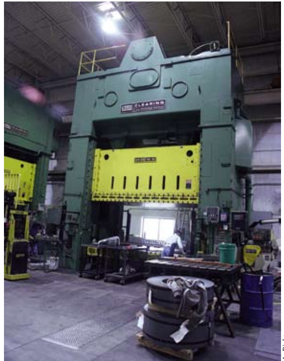
One of the larger mechanical presses that Walker Tool & Die uses to try out dies.
