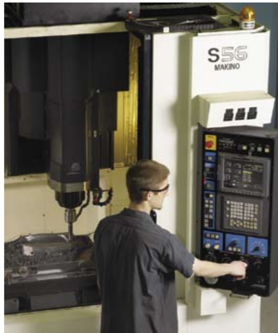
A Makino S56 vertical machining center is one of two Makino VMCs CAMmand uses for hard milling.
