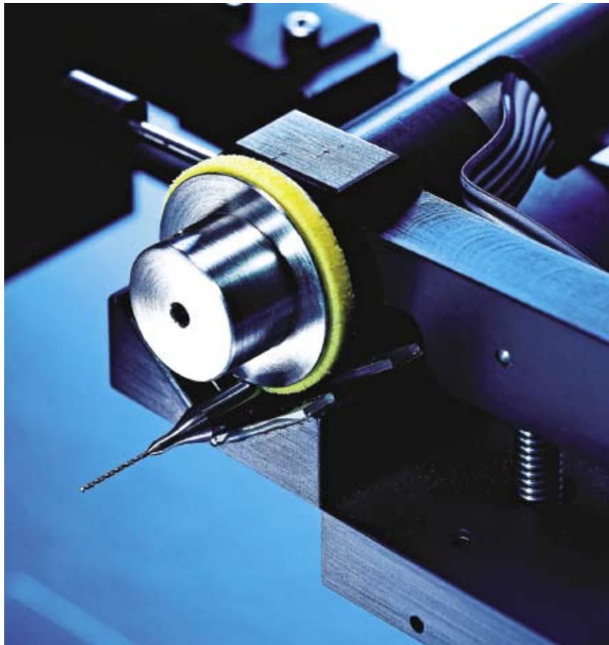
Measuring a microtool in a rotary V-block with zero runout.
