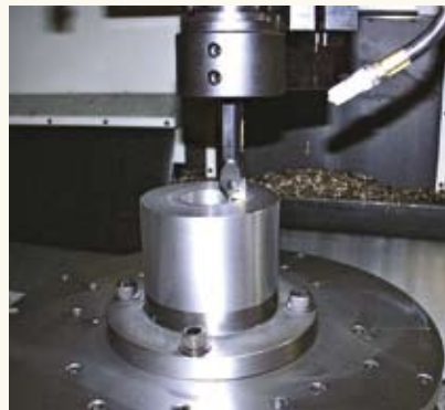
A high-precision mill/turn center turns the face of a mild-steel workpiece, which became part of an inspection gage inside another machine tool. The mill/turn center's design is based on jig machine tools, so it can perform precision work often done on jig borers and jig grinders. The machine also performed off-center precision boring and milling on the workpiece.
