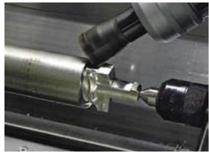
A multitasking machine tool processes a cylindrical bar, machining it into a turbine blade. Recent improvements to multitasking machine tools have included direct-driven assemblies and upgraded controls and memory.
