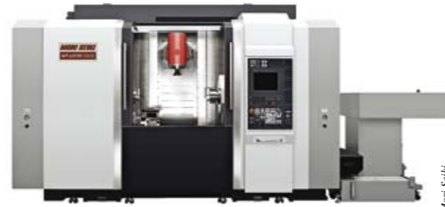
Consolidating turning and milling in one machine tool once involved noticeable compromising of one or both processes. But many mill/turn centers are designed today to be fully functional in their milling and turning.
