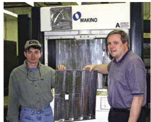
Phillip Jacobs (left) and Scott Smith of the University of North Carolina at Charlotte hold an aluminum structural panel for an aerospace application. Jacobs, who at the time was a graduate student, machined the structural panel at UNCC utilizing thin-wall milling.
