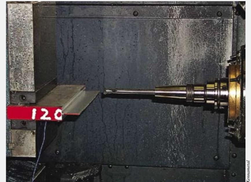
This test setup at Kennametal, featuring a ½"-thick aluminum plate machined using an endmill with its tool tip 10" from the spindle face, was designed to create exaggerated conditions that would clearly demonstrate the impact of changing variables in the machining system.
