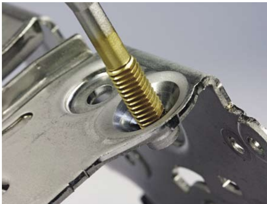
Although generally suitable for softer materials, some cold-form taps can tap materials with hardnesses up to 44 HRC.
