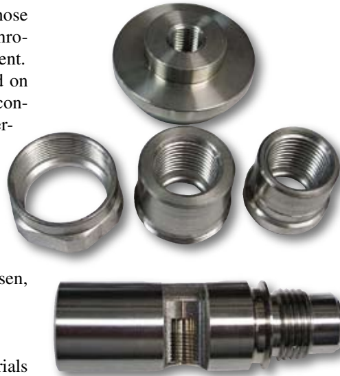
Taps can thread holes in a variety of materials, from aluminum to stainless steels (shown here) to materials with a hardness in the low 60s of the HRC range.
