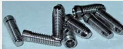
Magnetic finishers from Genevieve Swiss Industries are appropriate for deburring delicate parts, such as dental screws (bottom), while imparting a bright surface finish.
