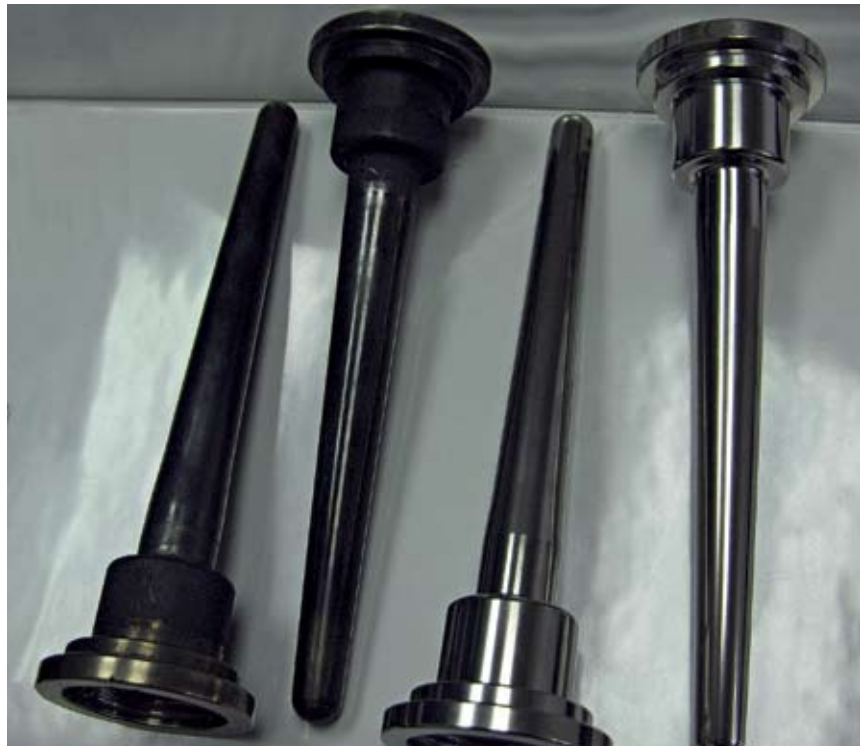
This series of mild steel plungers (used in the bottling industry) shows how microsurfacing progressively removes carbon deposits, enabling the parts to function significantly longer before requiring cleaning and maintenance.
