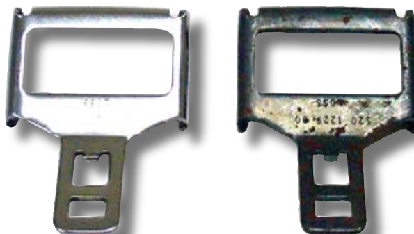
Before and after shots of a seat belt component that was microsurfaced.
