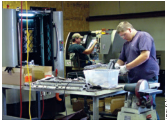
In Frog Legs’ “hybrid cell” are production manager Joel Farley (left) at an Amera Seiki TS-42 4-axis turning center, and Nathan Williams, assembly, at an Amera Seiki A-1 VMC. The cell arrangement gives Farley access to a variety of deburring and finishing equipment.
