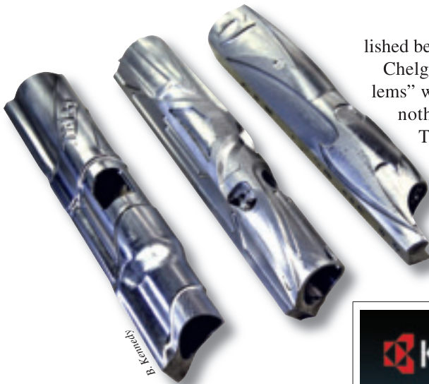
Three variations of paintball-marker body styles machined in "Op 2" at Smart Parts.
