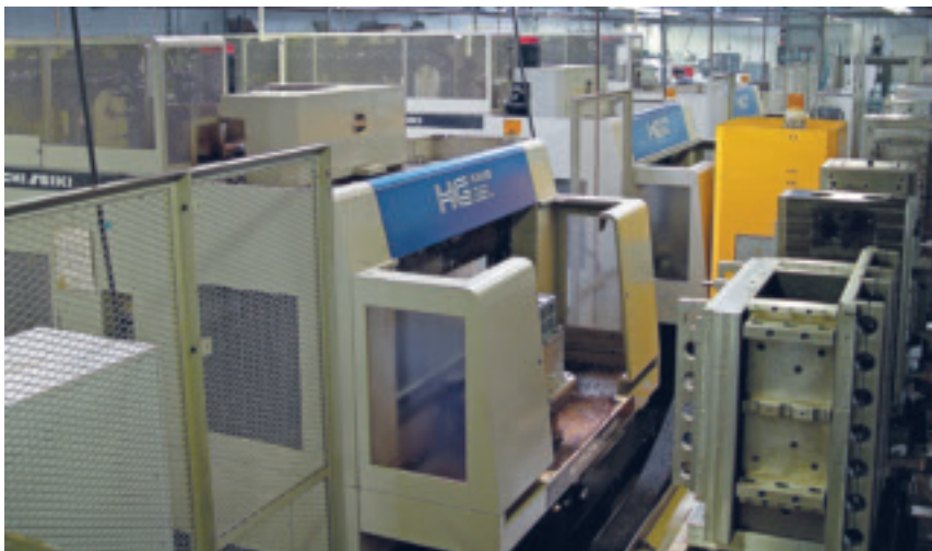
The largest cell at Morsch Machine consists of three Hitachi Seiki HMCs serviced by a rail-guided vehicle that handles 44 different pallets, each with a four-sided tombstone.
