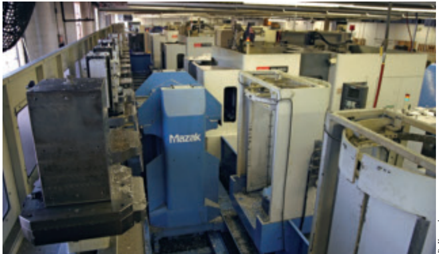
At Smart Parts, a rail-guided vehicle retrieves pallets from racks on the left, takes them to the loading station in the right foreground and then moves them between the three Mazak FH5800 HMCs.
