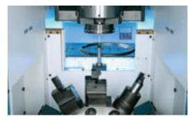
**EMAG LLC**, Farmington Hills, Mich., introduced the VSC vertical turning center for chucked components up to 340mm in diameter. According to the company, the machine tool is essentially a manufacturing cell, where the pickup spindle ensures the machine loads itself.
