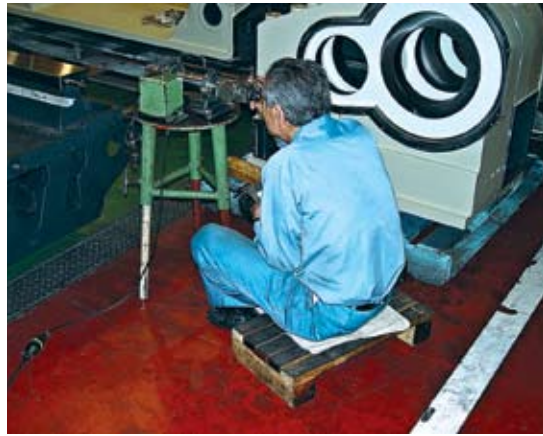
Technician measures flatness during machine tool production.
