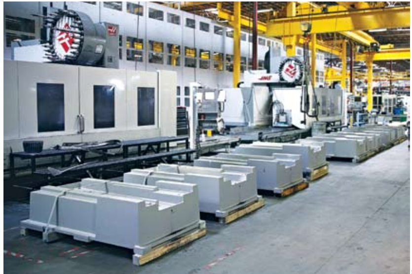
Extra-large specialty bed mill-type VS machines from Haas weigh from 60,000 to 75,000 lbs. and feature X-axis travels up to 150".
