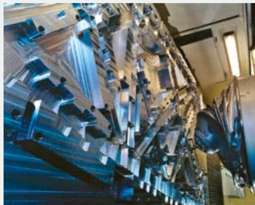
This Sprint Z3 parallel kinematic head at right from DS Technology is engineered with low mass to decrease acceleration forces in the X and Y axes.
