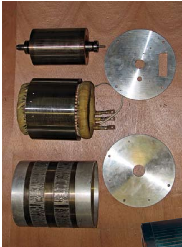
The 6"-dia, 10"-long rotor for the AC Propulsion motor, an assembly of copper and iron laminations, turns 13,000 rpm at the eBox electric vehicle's top speed of 95 mph.
