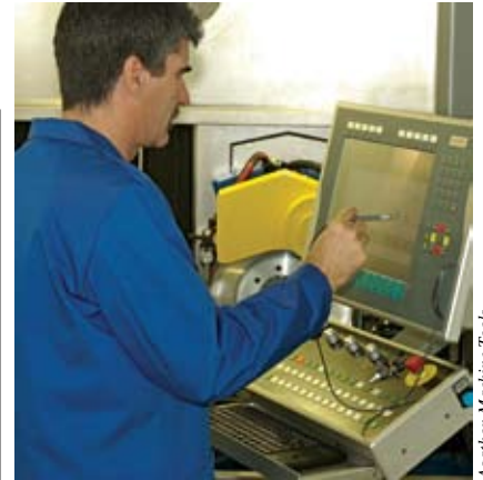
Agathon technician remotely accessing a machine tool via the Internet.
