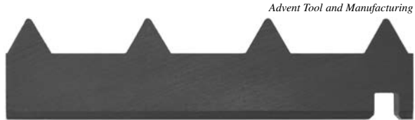
One option to minimize side-load pressure when thread milling long threads is to apply a skip-tooth form, such as one where every other tooth is missing.
