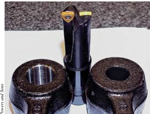
Powers and Sons uses CD 938 Coremaster core drills from OTM to open up 10.63mm- to 12.09mm-dia. cored holes (right) in forged and heat-treated 1541 steel idler arms. In a single pass, the drill takes the holes to within 0.5mm of finish size. The final diameter of 24.49mm, ±0.03mm (left), is then bored.
