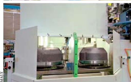
MAUS offers a frontal (top two images) or lateral pallet changer for loading and unloading parts.
