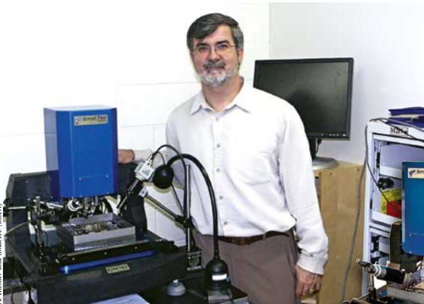
Jerry Mraz, general manager of SmalTec International, with the company's GM703 nanogrinding/microEDM machine. The GM703 has a 10-nanometer step resolution when mechanical micromachining and can generate a spark as small as 0.5µm when EDMing.
