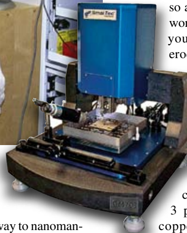
Jerry Mraz, general manager of SmalTec International, with the company's GM703 nanogrinding/microEDM machine. The GM703 has a 10-nanometer step resolution when mechanical micromachining and can generate a spark as small as 0.5µm when EDMing.
