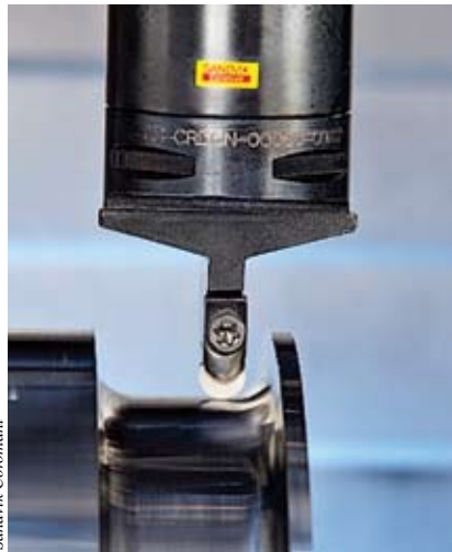
In 2007, Sandvik released two Sialon grades for machining nickel-base alloys.
