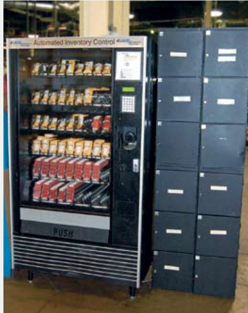
Automated vending systems include helical coil vending machines and automated lockers, such as these on Sealmaster's shop floor, and other types of systems, too.
