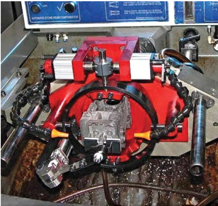
A die-cast, two-cycle chainsaw engine with an interrupted bore is chrome-plated and then honed to a 0.0002" tolerance on diameter, straightness and roundness.
