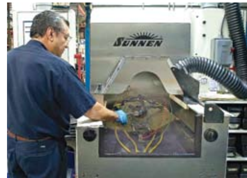
HydraForce operator setting up a Sunnen KGM 5000 Krossgrinding machine, which is used for finishing.
